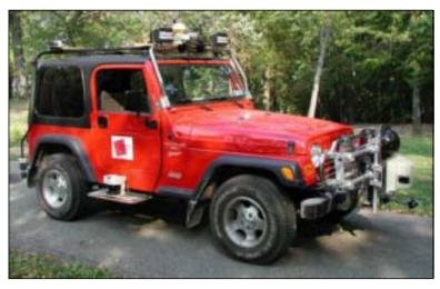
Fig 10. Autonomous Navlab; System for Intelligent Cruise Control
