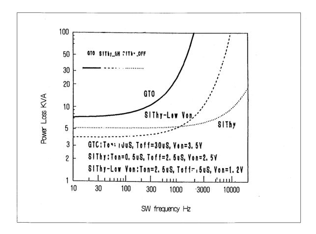
Our development was somewhat unexpected, that is, our device is capable of turning on and off the electricity with unexpectedly high efficiency. I would like to show you some data collected based upon this switching device that we developed.
