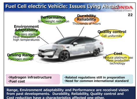
Fuel Cell electric Vehicle: Issues Lying Ahead. Range, Environment adaptability and Performance are received vision from past developments. Durability, Reliability, Quality control and Cost reduction have a characteristics affected one other. P-22
