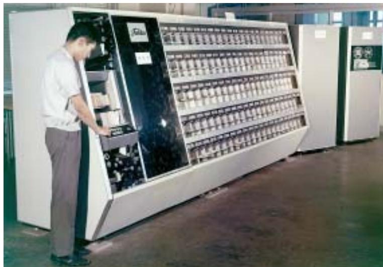
FIG. 1. Automatic reader / sorter of freely handwritten postal codes.
