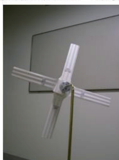
Micro Wind Turbine Rotor diameter: 200mm Materials: craft paper
