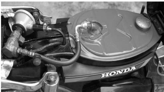
Fig. 8: LPG/gasoline bifuel tank components (a, b), Bifuel system set up (c) and LPG tank (d)
