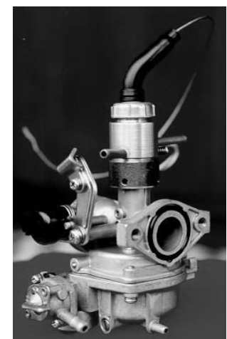
Fig. 6: LPG/gasoline caburettor with automatic obturating valve
