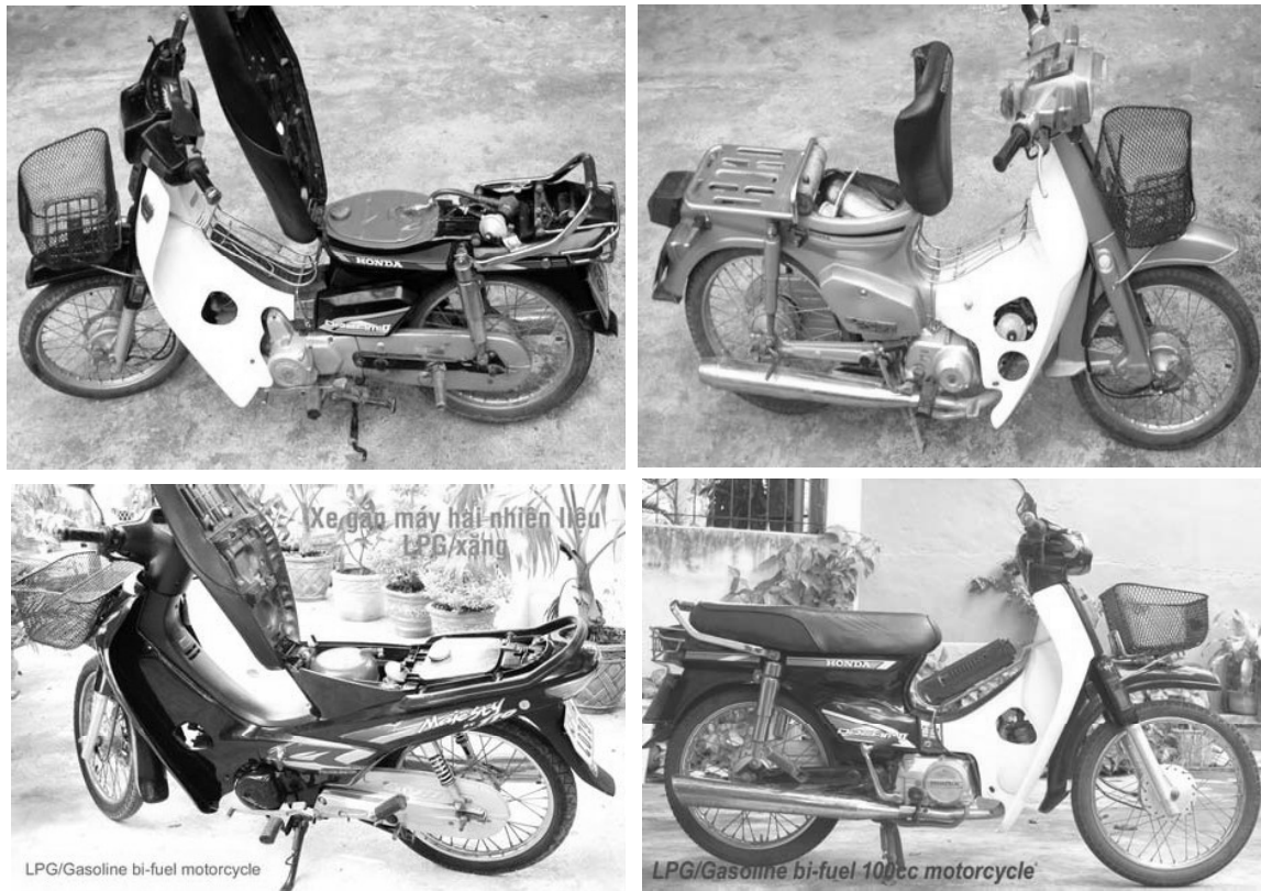
Fig. 9: Different possibilities of LPG/gasoline bifuel system installation on motorcycles
